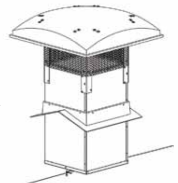
812240/812360 > Chimney Complete w/Dome, Bird Netting & Flashing
