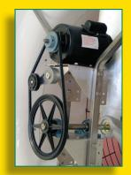
The orifice, blade, cone and motor combination optimizes the use of the motor's power curve.
