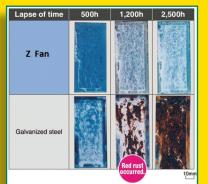
During a salt spray test, the Z-Fan housing and cone showed no signs of rust after 2,500 hours.
