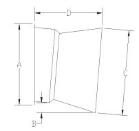
Rough Openings (H x W): SW = Slant Wall / D = Damper 36" SW - 44.5" x 43.5" / 48" SW/D - 55.5" x 55.5" / 54" SW - 60.25" x 60" / 54" D - 60.25" x 60.25"
