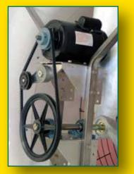
Motor mount and drive assembly utilize a rugged box frame design to increase motor life.
