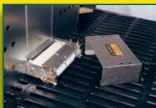
**Dual roller return idler assembly** at end of nest row provides adjustable belt tracking and brushes for belt cleaning.
