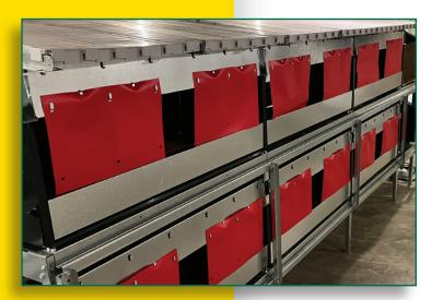
The 2-Tier Community Nest increases bird capacity within the same footprint (and can be wired into the same controls for ease of use!).
