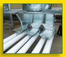
The Triple Upper Boot is designed to provide more feed to more flexible auger lines from one source. When used in conjunction with the double lower boot, up to six auger lines can run from a single feed bin!
