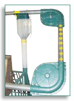
The Sure-Drop Model 780 Series Feed Drop installed on the Chain Disk Feed System
