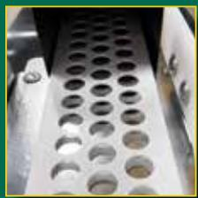
VAL-CO egg collection tables have a heavy steel construction – the toughest in the industry, with cast iron bearings, large utility shelf and a standard light fixture – and easy access to the direct drive and egg belts for maintenance and cleaning.
