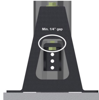
Figure 5: Leave 1/4" (+/- 1/8") gap between C-channel and bracket.
