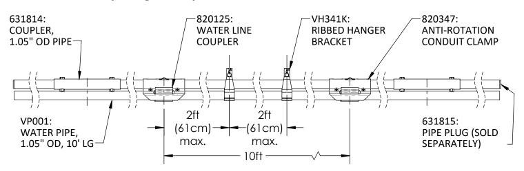
SUPPORT EVERY 8'-10', EITHER FROM WRAPPING AROUND STEEL PIPE, OR DIRECTLY FROM STEEL BRACKETS (P/N 820347 OR 820387).
