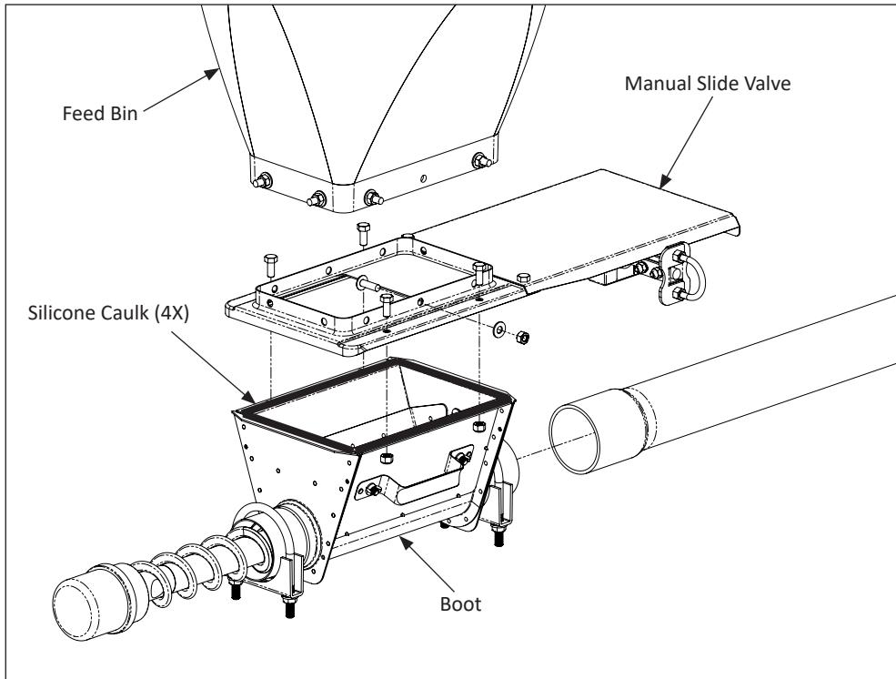
**NOTE:** If using a restrictor plate (such as 730875), install the restrictor plate between the slide valve and boot.
