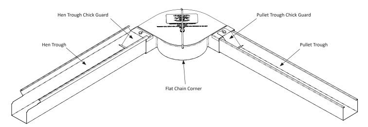
**NOTE:** The Corner Chick Guard (*Pullet Trough*: **410597** and *Hen Trough*: **410598**) is only designed to be used on VAL-CO flat chain corners.
