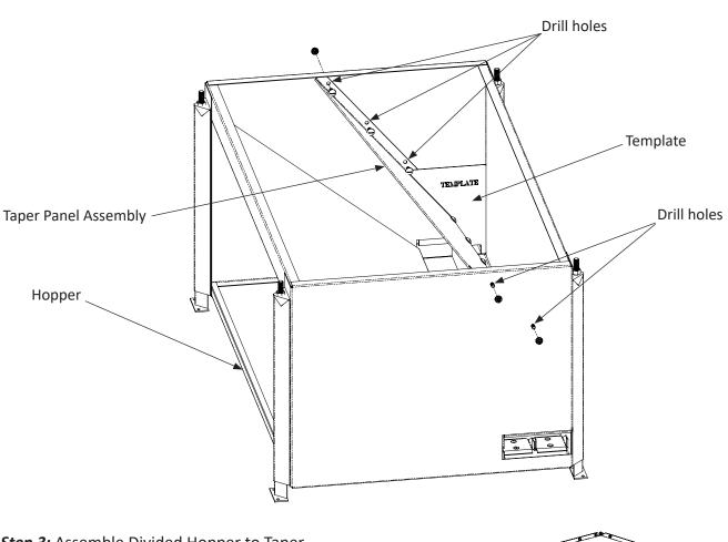
Step 3: Assemble Divided Hopper to Taper
