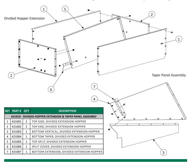
**Step 2:** Use provided Template to locate Taper Panel Assembly inside Hopper and then use pre-drilled holes in flanges of Taper Panel Assembly to mark holes to be drilled in Hopper. Use 3/8" drill bit. Assemble Taper Panel Assembly to Hopper using 5/16-18 Truss Bin Bolts and 5/16-18 Hex Flange Nuts, as shown below.
