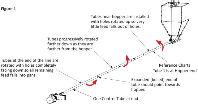
1. Loosen the tube clamps, or if the line is new, leave the tube clamps loose until the line has been programmed. BE SURE TO TURN OFF ALL POWER BEFORE SERVICING!
