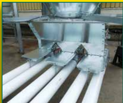
The Triple Upper Boot is designed to provide more feed to more flexible auger lines from one source. When used in conjunction with the double lower boot, up to six auger lines can run from a single feed bin!
